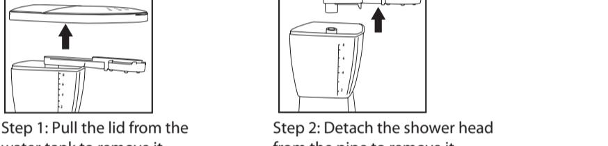
Step 1: Pull the lid from the water tank to remove it.
